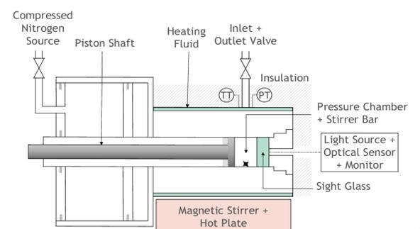
Figure 1: HPBDP Experimental Setup
