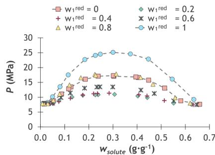
Figure 3: HPBDP Data at 308.2 K for Different Solvent-Free 1-Nonanol Fractions ( $w_1^{red}$ )
