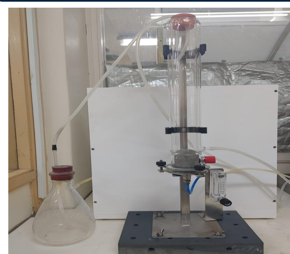
Figure: Ion/Precipitation flotation column with heating jacket and additional vacuum pump and beaker for froth removal.
