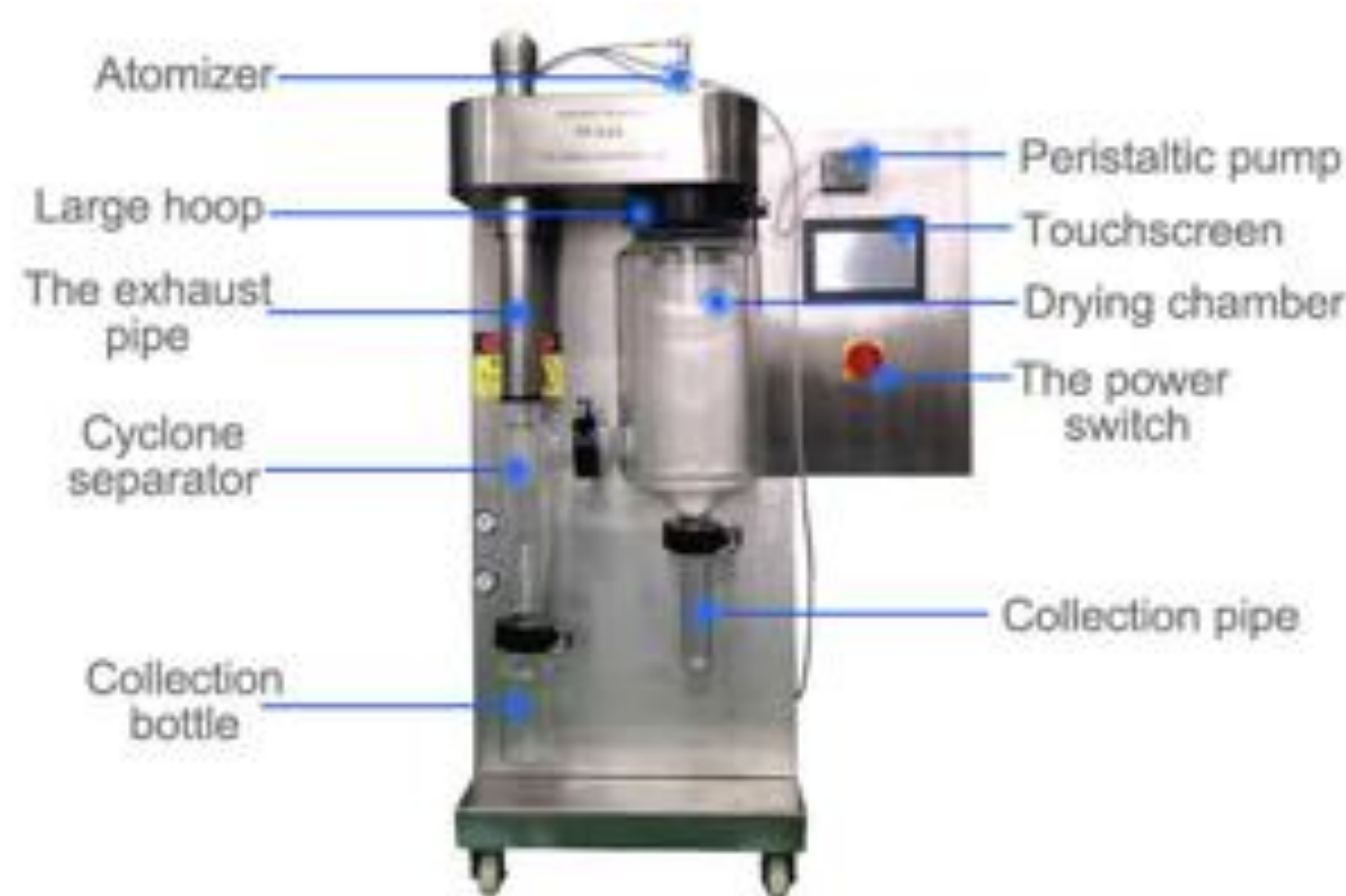
Figure 2 Schematic of a laboratory spray dryer.
